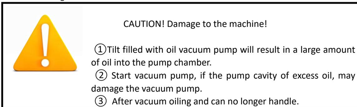
Note: Before transporting the machine, make sure that the vacuum pump oil drained.
